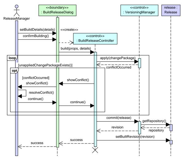
Figure 4.8.: Dynamic behaviour of the Build Release use case
