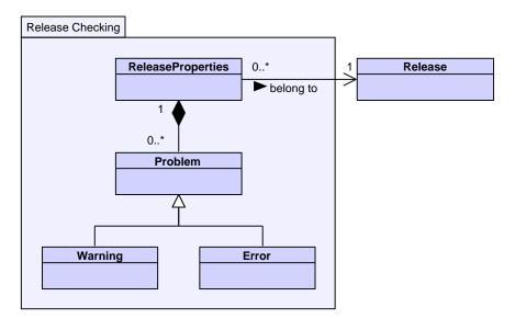
Figure 4.3.: The entity classes of the release checking package
