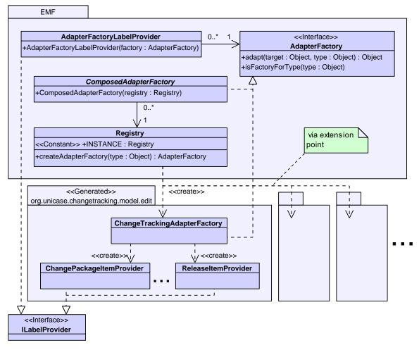
Figure 6.5.: Classes for using EMF label providers
