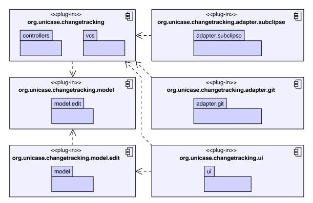
Figure 5.2.: The plug-ins of the prototype
