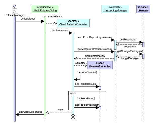
Figure 4.7.: Dynamic behaviour of the Check Release use case
